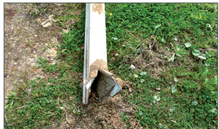
Picture 4: Destroyed by obstacle - ramming profile during testloading feasibility study
