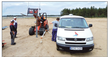
Pict. 3: Testloadings on mini steel piles on a 62 MWp PV - park
